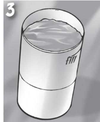
3. Fill the jar to the turbidity line located on the label.
