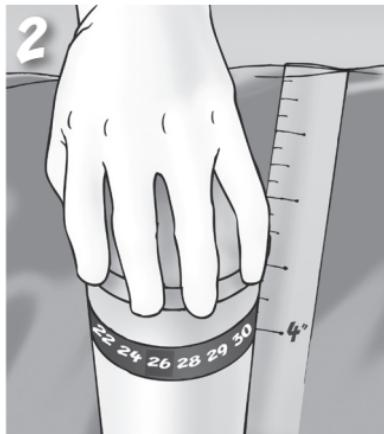
2. Place the thermometer four inches below the water surface for one minute.
