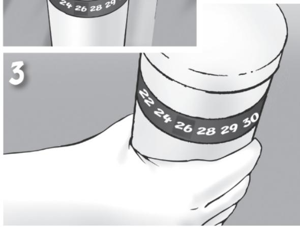
3. Remove the thermometer from the water, read the temperature and record the temperature as degrees Celsius.
