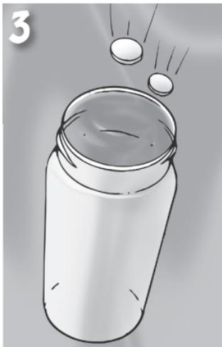
**3.** Drop two Dissolved Oxygen TesTabs® (3976A) into the vial. Water will overflow when the tablets are added.
