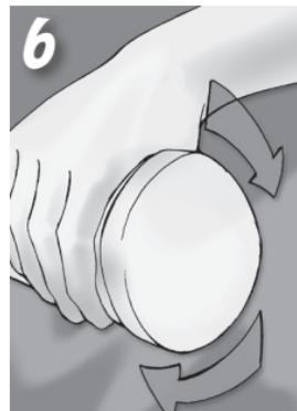
**6.** Cap the full jar while it is still submerged. Remove it from the river immediately.
