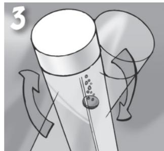
3. Cap and mix by inverting until the tablet has disintegrated. Bits of material may remain in the sample.
