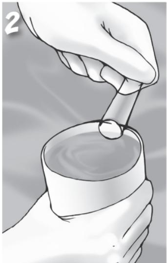
**2.** Submerge the small vial (0125) into the water sample. Carefully remove the vial from the water sample, keeping it full to the top.
